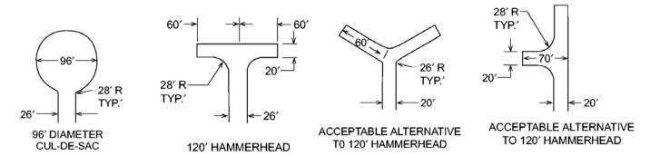
**3.10.1 Cul-de-sacs-** Cul-de-sacs shall have a clear and unobstructed turning radius that is consistent with the capabilities of the fire apparatus of the local fire department and not less than 96 feet in diameter, subject to approval by the fire code official.
